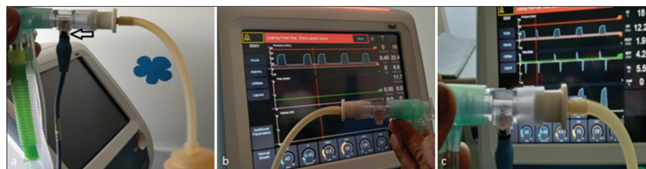
Figure 1: (a)The flow sensor-heated wire anemometer is a data link between the patient and the machine (arrow). (b)The monitor shows the pressure-time curve only when the sensor is not attached. (c)With an intact sensor, the flow and volume curves are also seen.
